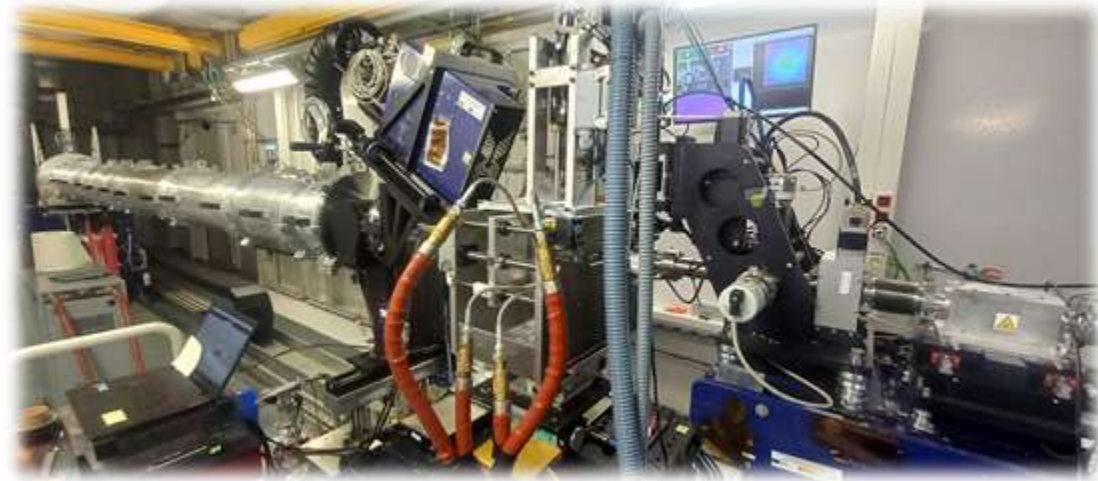
Figure 5 A photograph of the operando X-Ray Scattering Injection Moulding Stage mounted on the NCD-SWEET beamline at the ALBA synchrotron light source.
